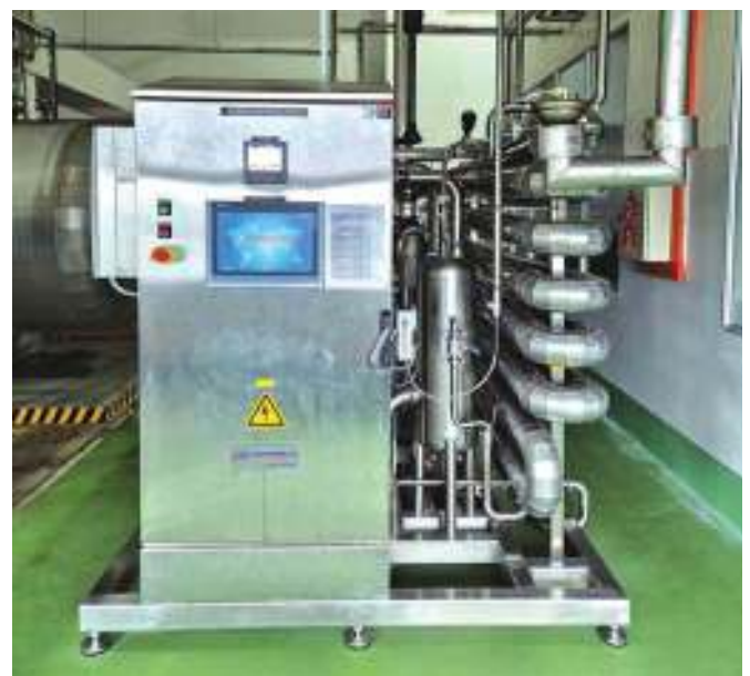
HTST (High Temperature Short Time) system in Singapore plant
